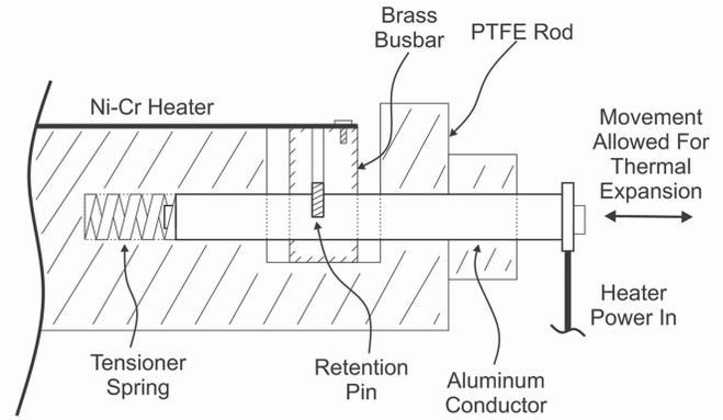
Fig. 5. Heater strip tensioning system used in the design.
