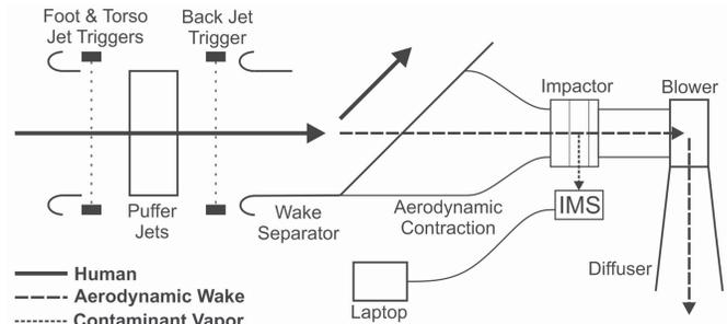
Fig. 1. Schematic of the wake sampling portal.
