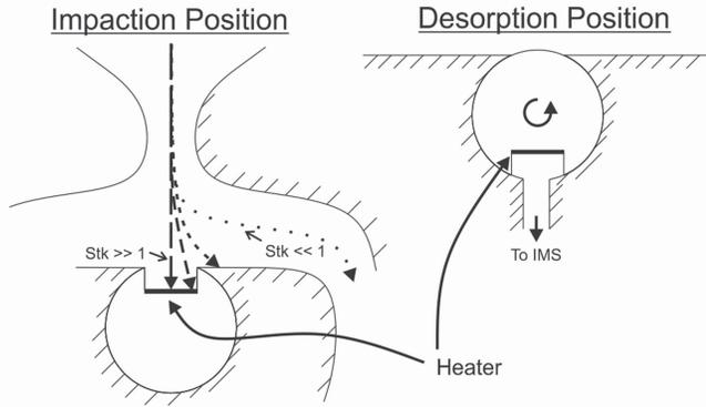
Fig. 4. Schematic showing the operation of the rotating rod with heated impaction surface.
