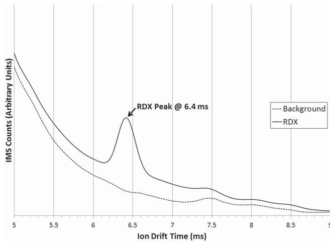
Fig. 6. IMS output plots showing RDX peak visible against background signal.
