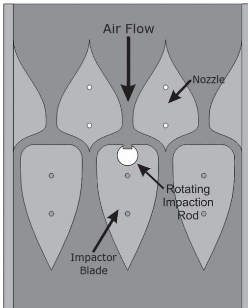
Fig. 3. Top down view of the impactor section geometry.
