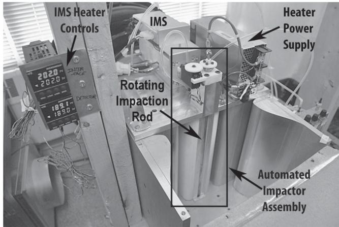
Fig. 2. Completed impactor assembly with integrated desorption and sampling. Impactor nozzles in front of instrumented blade have been removed to show the rotating impaction rod and heater strip.
