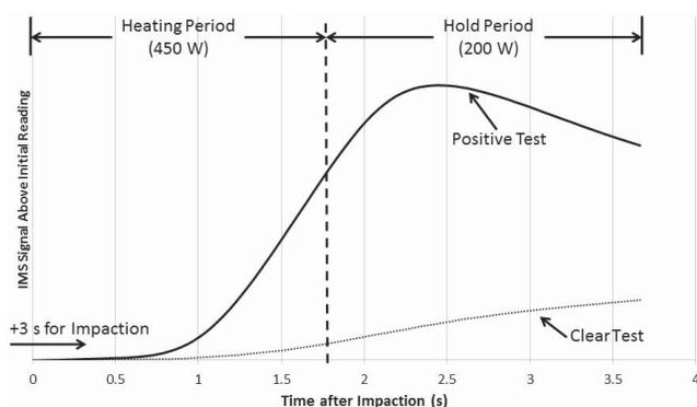
Fig. 8. Signal timelines for explosive-laden and clear patches applied to the torso, showing positive tests peaking and rolling off before the end of the interrogation period.
