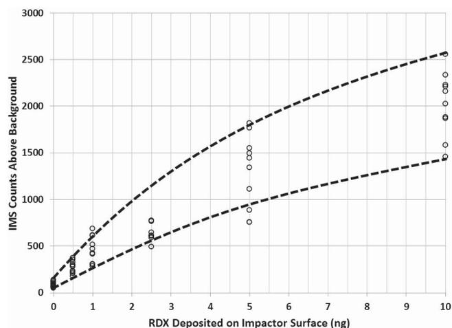
Fig. 7. Calibration curve for IMS used to check day-to-day results. Dashed lines: acceptable range of signal.
