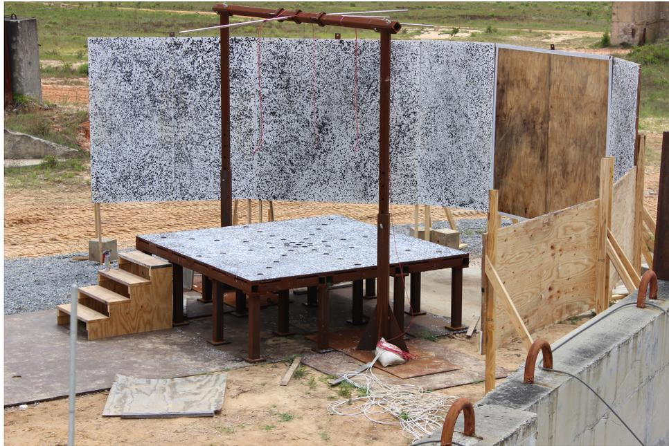
Figure 6.2: Photograph of part of the setup for the large scale tests. In the center of the image is the reflection platform in which the starburst pattern of the pressure gauges can be seen. The speckle boards used as a background for BOS are positioned behind the reflection platform. The non-speckled space is where the retro-reflective shadowgraph screen is placed prior to the test.
