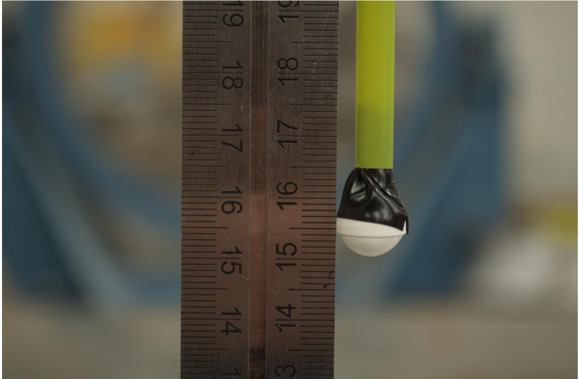
Figure 4.2: A PETN pellet with an RP-3 detonator attached to it with electrical tape. The pellet is suspended over the test section. The yellow tube above the charge is a polymer straw used to provide a consistent charge height. A ruler with cm graduations, used to determine the exact charge height, is shown to the left of the charge.
