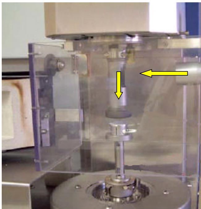
Figure 2: UV-Curing device based on ARES unit
