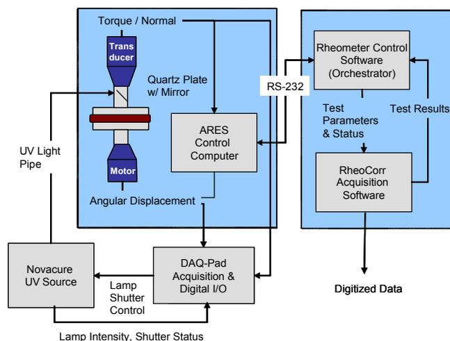
Figure 1: Experimental setup with fast data acquisition and UV curing option
