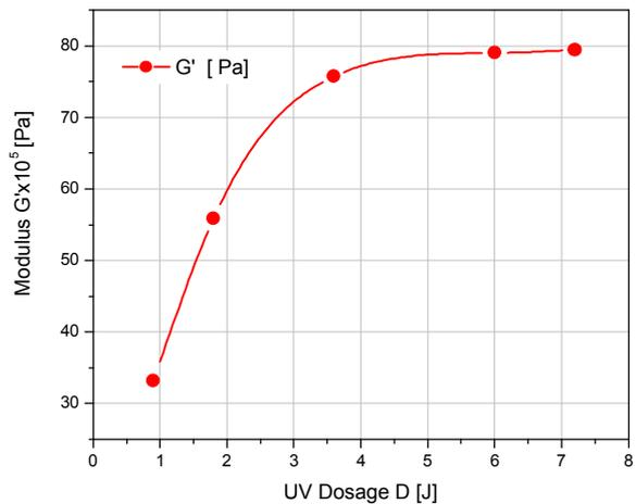
Figure 8: The influence of UV exposure dosage to the material's final modulus
