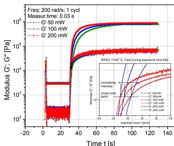
Figure 5: Influence of ultra-violet light intensity to the curing reaction. Sample modulus vs reaction time at different UV intensities
