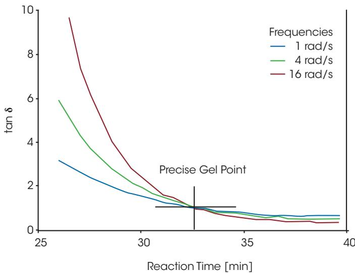
Figure 5. The gel point identified by the intersection of  $\tan \delta$  curves generated from the simultaneous frequency sweeps
