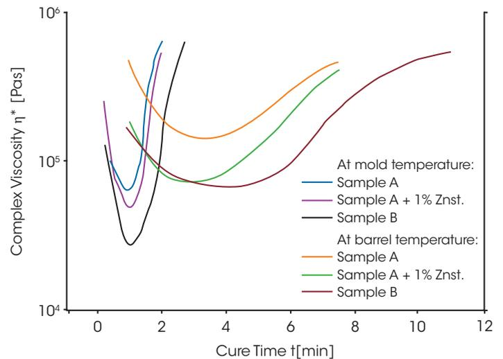
Figure 9. Effect of Zn stearate on the viscosity profile during cure at barrel and mold temperature
