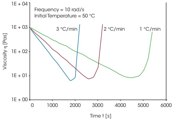
Figure 6. Measurement of the viscosity profile of an epoxy resin as a function of the heat-up rate
