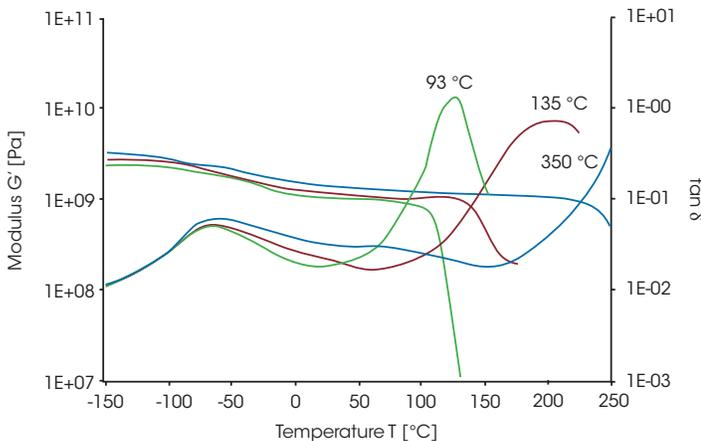
Figure 8. The extent of the cure of a thermoset as a function of the curing temperature shows in  $T_g$
