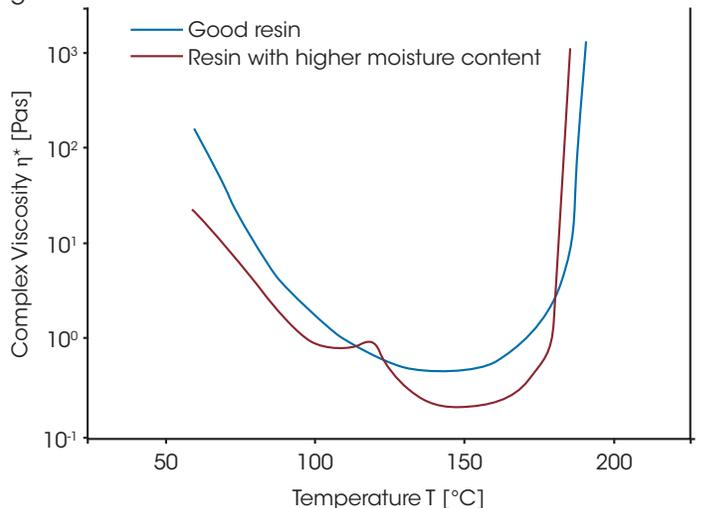
Figure 7. Viscosity as a function of temperature for a good and a bad (excess moisture) sample
