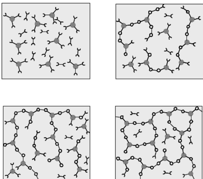
Figure 1. Schematical representation of structural development during thermoset curing for the reaction of a dimer with a trimer
