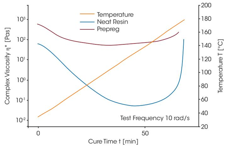
Figure 11. Viscosity profile of composite (prepreg) and the neat resin during cure
