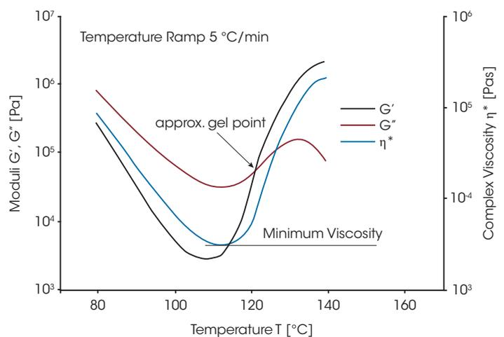
Figure 3. Measurement of the minimum viscosity and approximate gel point for a curing epoxy compound
