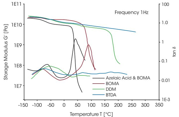
Figure 10. Effect of different curing agents on the mechanical properties of the final product
