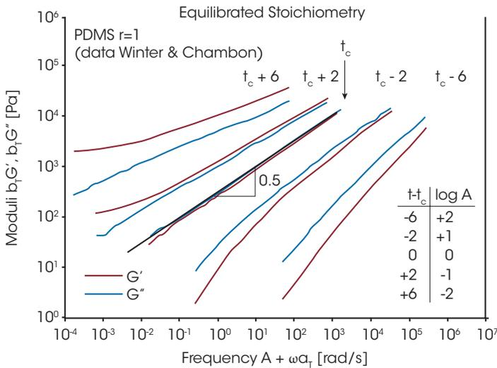
Figure 4. Frequency sweeps measuring  $G'$  and  $G''$  at any point in time during cure
