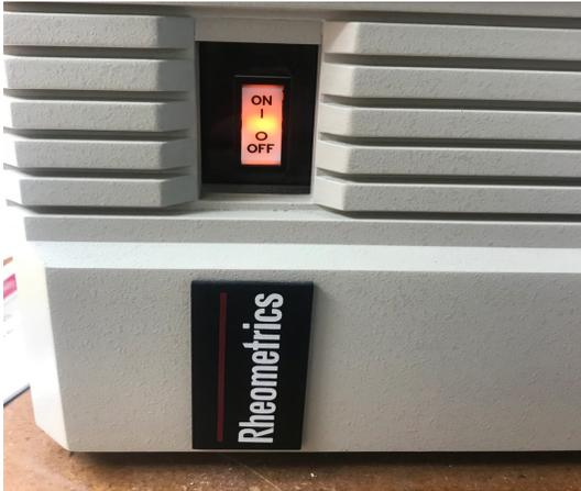
*The on/off switch on the side of the ARES*
