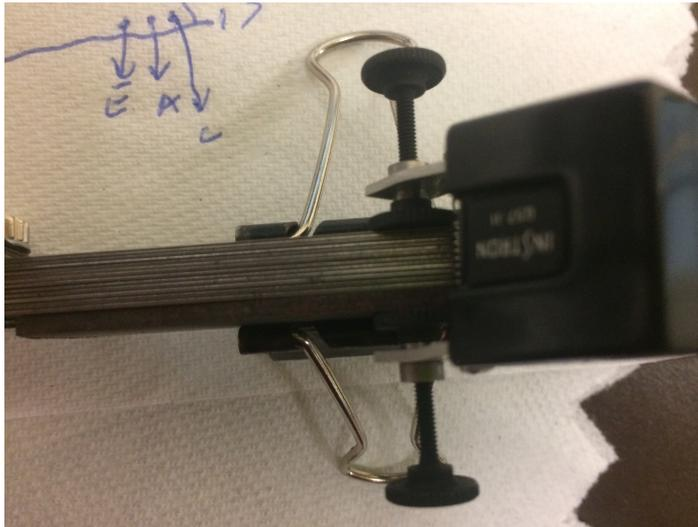
2) Additional 1 metal strip of Feeler gauge measured with caliper (0.022 inches)
